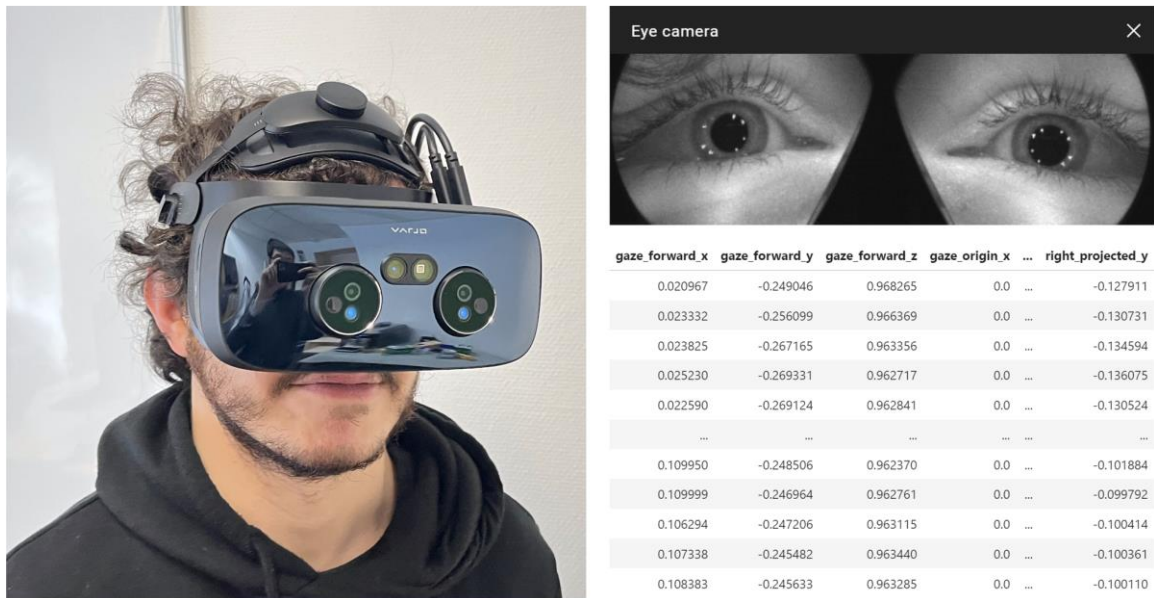
Figure 9 Left: Varjo XR-3, which is a high-end HMD device for both VR and AR. Upper right: eye images taken by cameras inside Varjo XR-3. Lower right: some eye features recorded by Varjo XR-3 (Bozkir et al., 2023).
